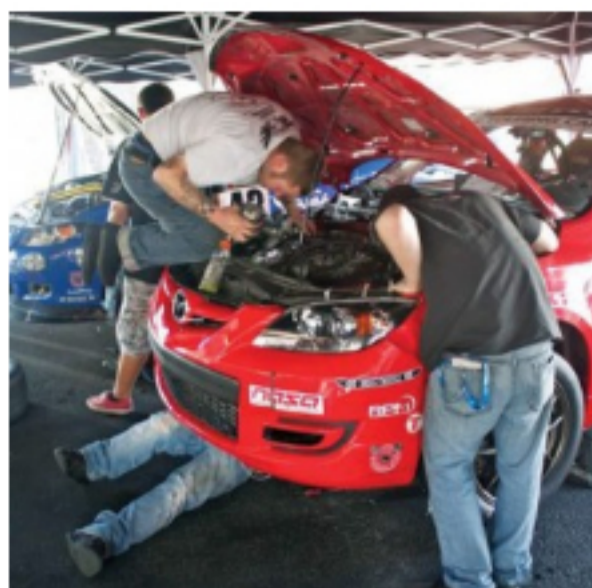
AJ Gracy, of Performance In-Frame Tuning, gets on top of the engine of the No. 3 car while Drew Ferneau works underneath to replace the turbo with only minutes to spare before the race begins. Victor Martinez photo
